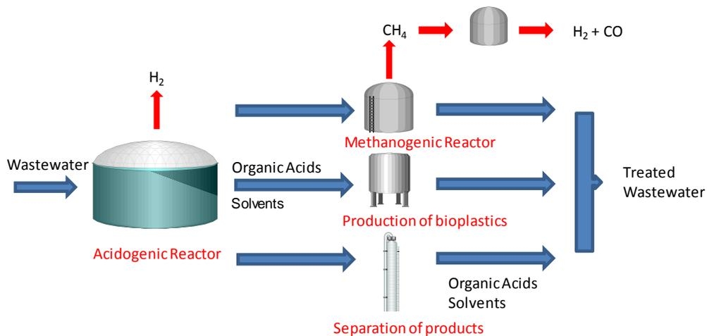
Anaerobic reactors are a core technology in a wastewater treatment plant as the process generates a broad spectrum of organic acids and solvents in the liquid phase besides hydrogen and methane in the biogas
